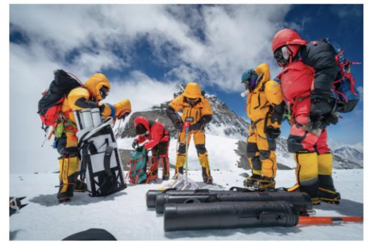
Researchers drill the highest ice core ever recovered at 27,000 feet elevation with the summit of Mount Everest in the background. (Image credit: Dirk Collins, National Geographic)
